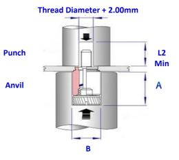
Punch Or Drill Hole To Specified Diameter (DO NOT Deburr The Hole Seat Fastener Squarely In The Hole Squeeze Fastener Into Panel Until Shoulder Of The Fastener Makes Contact With The And No Serrations Are Showing
